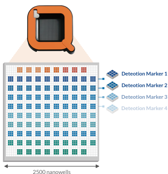
Figure 2. Schematic diagram of PanelChip® and its specifications.
